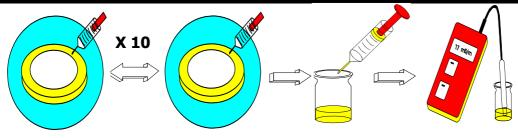
Leave water inside for 1 minute (NB 1'st time only) Retrieve water back into syringe. Last time as much as possible Remove syringe and empty back into the original beaker Measure conductivity of the approx 10 ml in the beaker in  $\mu$ S/cm **Result = A**
