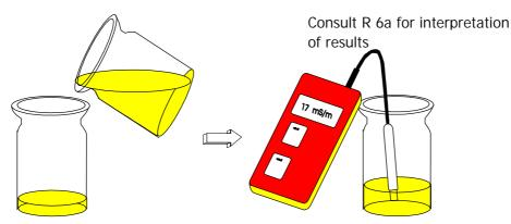
**DECANT into CLEAN GLASS** JAR washed with destilled water and dried out.
