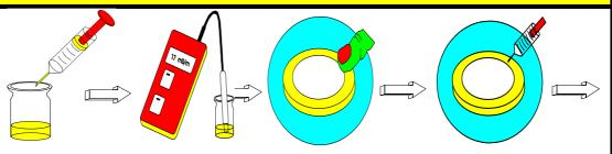
Fill in 10 ml distilled water into clean beaker using the syringe, ie. 2 x 5 ml
