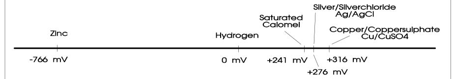
When testing and specifying HEMPEL - unless otherwise appearing - use and refer to the saturated Calomel reference anode as basis.
